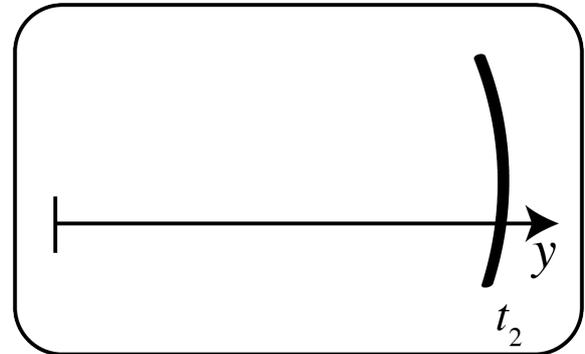
Measurements of the y position at two times, and the difference in the times allow calculation of the speed.
