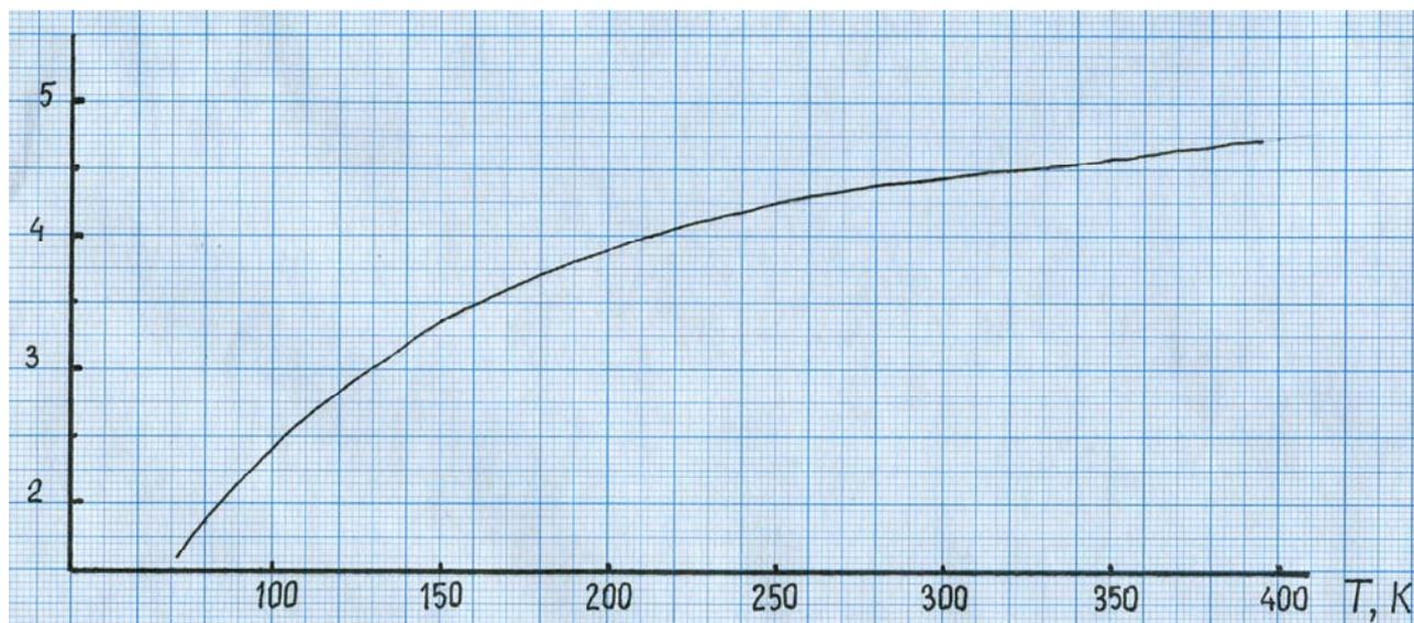
Fig. 1. The relationship between aluminum's specific heat in arbitrary units and temperature.
